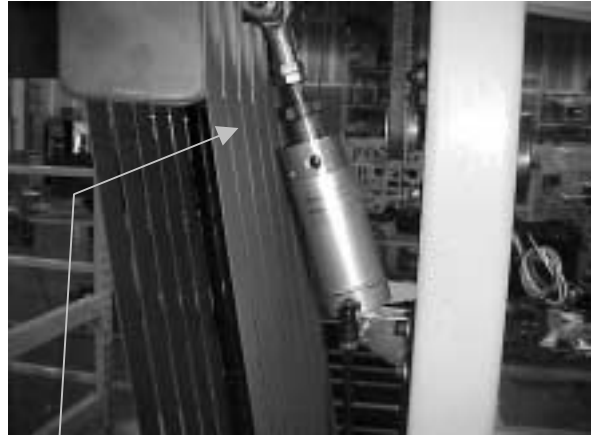
Above view shows the set collar that sets the gap shown at the left
