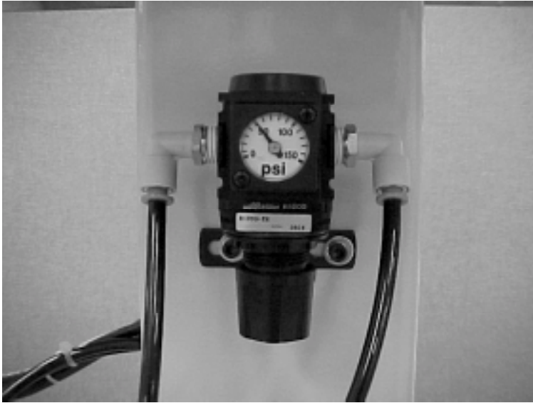
Drape Table Air Pressure Regulator. Set at 50 psi.
