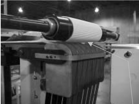
Above view shows the correct gap between the 1" belts and the top
