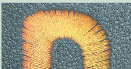
When using a cutting point on embroidery, lengthways and across the grain, the cuts in the leather are different. In extreme cases, the design can be completely cut out from the leather.
