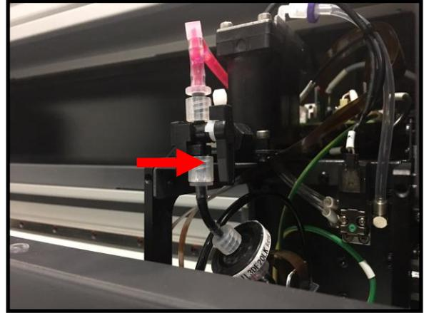
Move the bottom manual 3 way valve so it is in the 9:00 (9 o'Clock) position. This will let the ink flow through the purge line.
