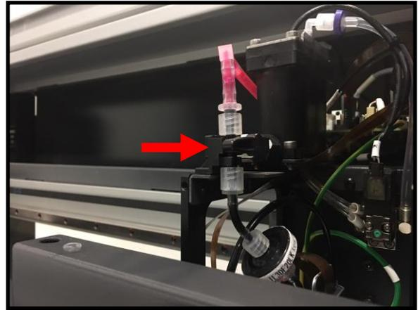
Move the bottom manual 3 way valve so it is in the 9:00 (9 o'Clock) position. This will let the pink flushing solution flow through the purge line and evacuate the ink that is in place.
